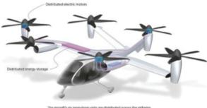
Each of these units is connected to two separate batteries.
