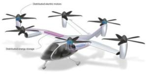
The aircraft's six propulsion units are distributed across the airframe Earth of these units is connected to two separate batteries.
