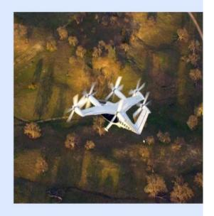
When flying overhead, the aircraft registered 45 A-weighted decibels (dBA) at an altitude of 1640 feet (500 meters) at 100 knots airspeed, and during planned take-off and landing profiles it measured below 65 dBA at 330 feet (100 meters) from the flight path. In other words, the aircraft will barely be perceptible from the ground when flying over a typical urban environment and guieter than a conversation when taking off and landing.
