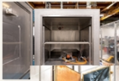
Battery in altitude chamber
