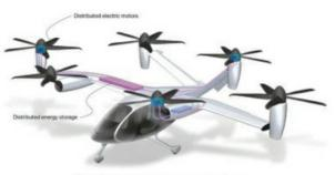
The aircraft's six propulsion units are distributed across the airframe. Each of these units is connected to two sensate batteries
