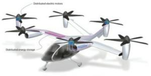
The aircraft's six propulsion units are distributed across the airframe Each of these units is connected to two separate batteries.
