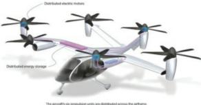
The aircraft's six propulsion units are distributed across the airframe
