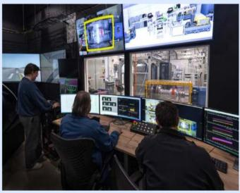
The ITL will support activities across our certification and test program, including safety-of-flight testing for the first aircraft to roll off our production line. It will also play an integral part in preparing for flight with a pilot on board and be validated by the FAA as a conforming test facility, capable of running for-credit tests at all hours of the day as part of our ongoing certification program.
