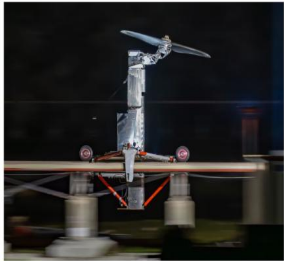
Our 'Whirly' propulsion system test asset, used to conduct endurance testing.
