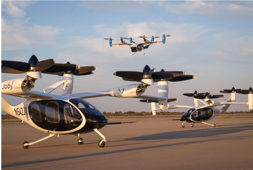
Two of Joby's battery-electric production prototype aircraft in Marina, California, with the company's hydrogen-electric technology demonstrator in flight above. Joby Aviation Photo
